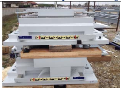
Lyon Stadium - General View –Spherical bearings between metallic pier and concrete support
